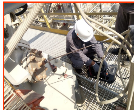
Stack Emission Testing
